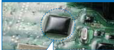
Computer control board surface adopting SMT packaging technology
